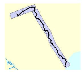
To create a linear index layer you must first select a linear feature to create an index for and then select **Tools**\Create Linear Index Layer... from the MapLogic Layout Manager toolbar.
