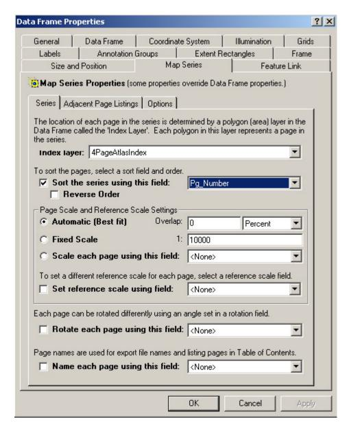
The above example displays the properties of a map series frame. You will notice that the element will have all the normal properties you would expect for that type of element with an added tab for properties specific to our extension. Modify the element properties just like you would with any other element in ArcMap.
