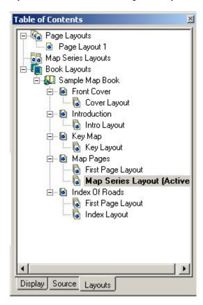
The Layouts tab is a new tab that is added to the ArcMap Table of Contents by the *MapLogic Layout Manager*. If the Layouts tab is not visible after you install the extension, you can make it visible by selecting Tools>Options... in ArcMap's main menu. Go to the TOC tab, make sure Layouts is checked and press the OK button.
